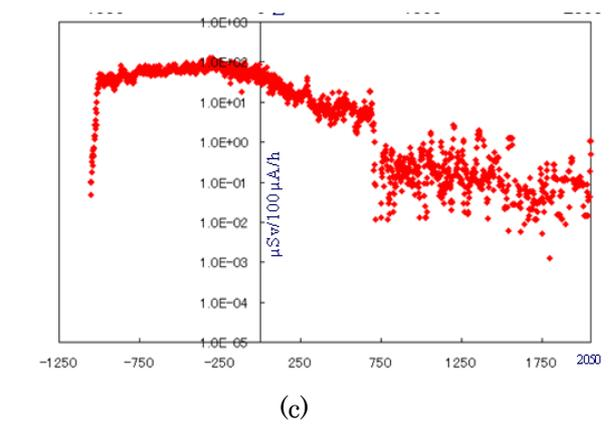
Fig. 7 Neutron equivalent dose distribution for whole domain: (a) two dimensional distribution of top view; (b) Y=0 (c) Y=300 cm
