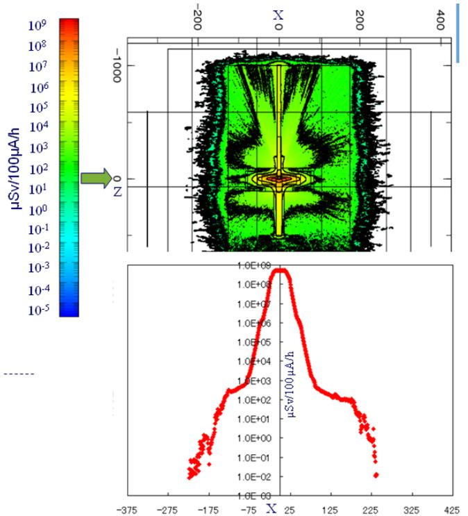
Fig. 13 Neutron equivalent dose distribution for whole domain: (a) two dimensional distribution of side view; (b) Z=0 cm
