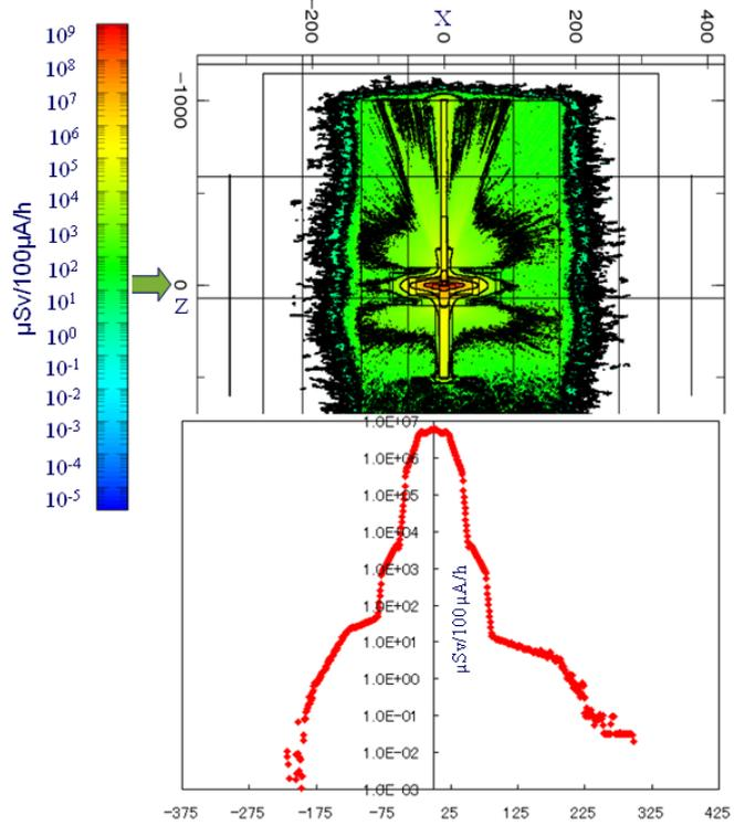
Fig. 12 Photon equivalent dose distribution for whole domain: (a) two dimensional distribution of side view; (b) Z=0 cm
