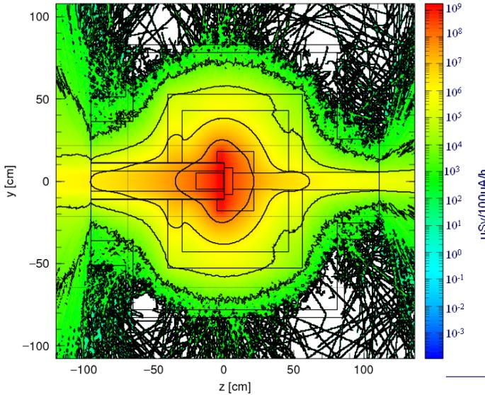
Fig.3. Neutron equivalent dose distribution around target station
