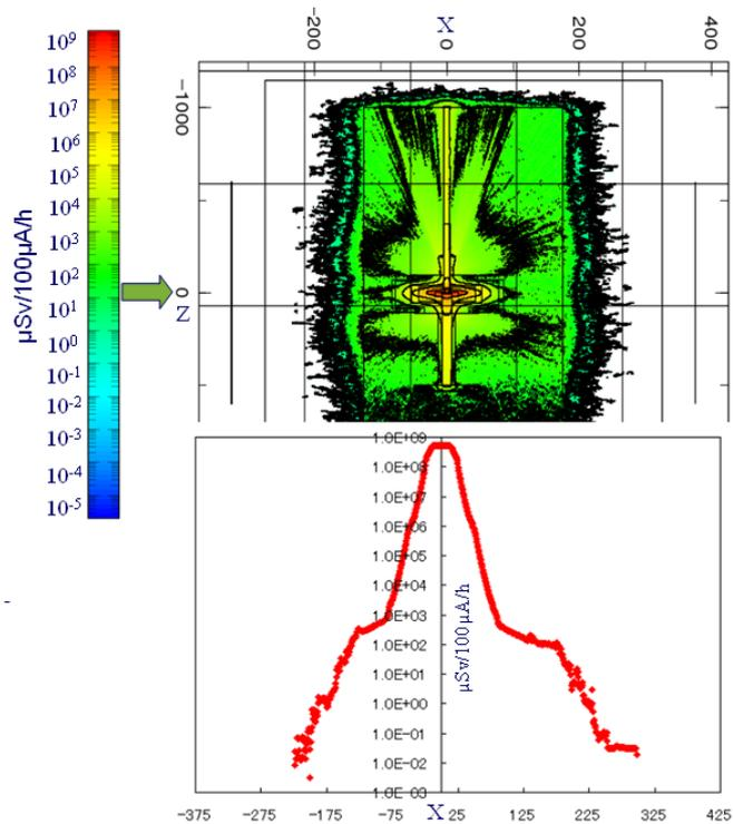
Fig. 14 Neutron+Photon equivalent dose distribution for whole domain: (a) two dimensional distribution of side view; (b) Z=0 cm
