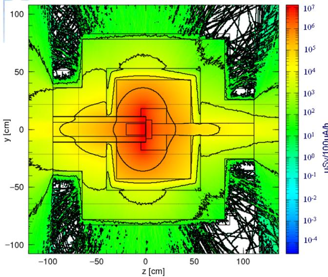
Fig.4. Photon equivalent dose distribution around target station
