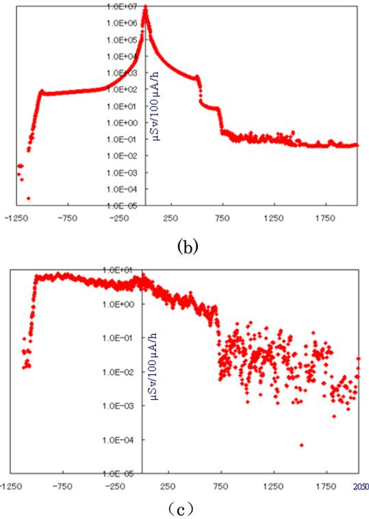
Fig. 6 Photon equivalent dose distribution for whole domain: (a) two dimensional distribution of top view; (b) Y=0 (c) Y=300 cm
