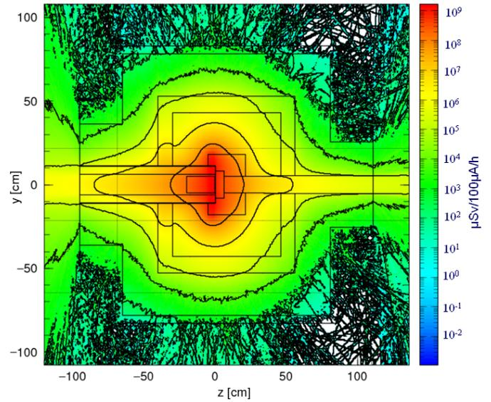
Fig.5. (Neutron+Photon) equivalent dose distribution around target station
