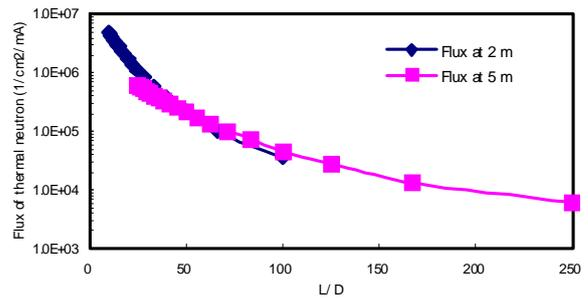
Fig.5. Flux of thermal neutron according to the L/D, (moderator material: polyethylene, moderator thickness: 5 cm)
