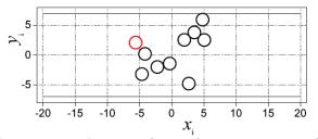
Figure 3. A snapshot showing a single microswimmer (red circle) propelling in a channel in presence of low-density passive particles. The motion of the microswimmer in this case is similar to that of a free microswimmer but with re-normalized self-propelled velocity and the mobility of passive particles.
