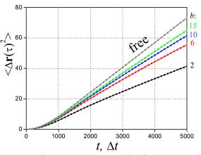
Figure 2. The mean square displacement of a microswimmer for channels of various widths:  $d/(2r_0) = 2, 6, 10, 15$  and for a free particle in 2D.
