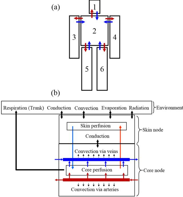
Figure 1. Schematic representations of (a) six-cylinder model of the human body (1, head; 2, trunk; 3, right upper extremity; 4, left upper extremity; 5, right lower extremity; 6, left lower extremity) and (b) the core and skin nodes and their interactions with CVS and external thermal environments.
